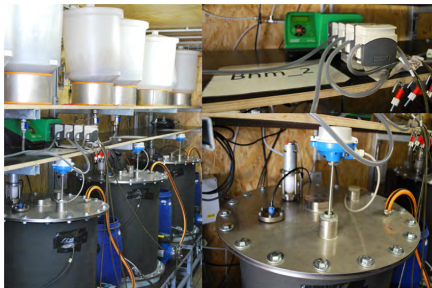
Fixed-bed reactors with feeding pump for biological methanation
