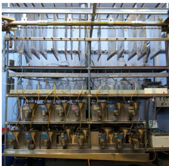
CSTR lab.-scale system used for the research on nitrogen
