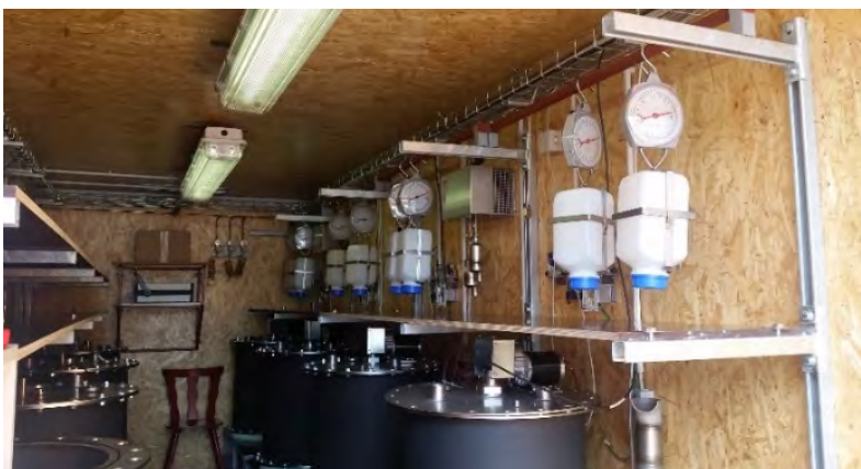
Laboratory container for hydrogen injection experiments
