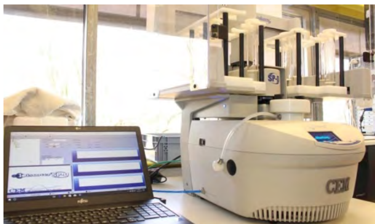
The new device for microwave digestion of samples for determination in ICP-MS
