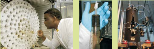
Hohenheim Biogas Yield Test (left) High Pressure fermentation (right)
