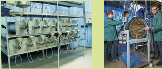
Horizontal Digesters for Semi-Continuous and Batch-mode (left) / Two-phase anaerobic digestion (right)
