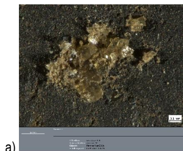
MAP on the cathode surface after BES treatment (a) and experimental setup for CO 2 treatment of digestate (b)
