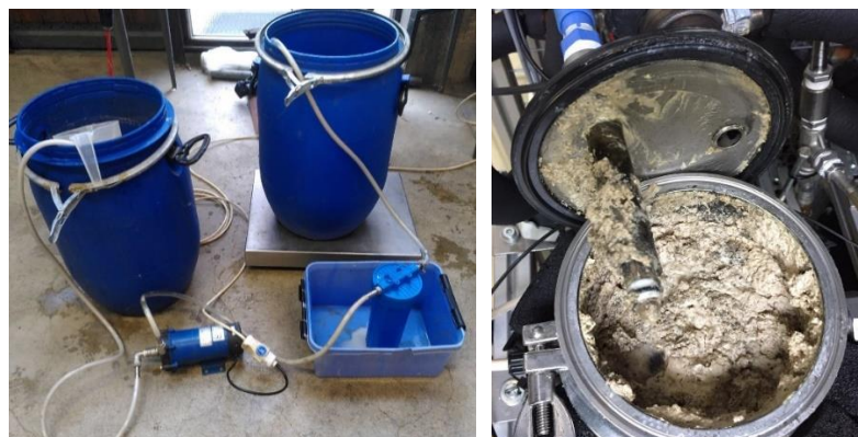
Substrate preparation, i.e. filtration of the dairy wastewater (left) and deposition of undegraded substances on the liquid surface of the reactor (right)
