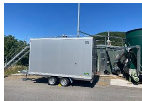
Measurement of gas components directly at the fermenters with new sensor technology. The installed UV spectrometer can be seen on the right
