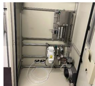
Measurement of gas components directly at the fermenters with new sensor technology. The installed UV spectrometer can be seen on the right
