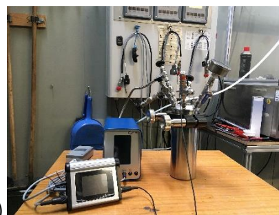
MAP on the cathode surface after BES treatment (a) and experimental setup for CO 2 treatment of digestate (b)
