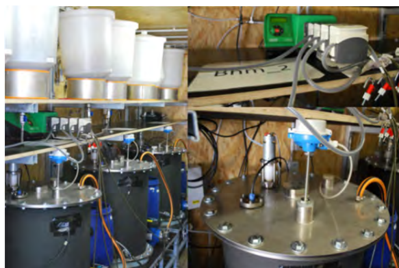
Fixed-bed reactors with feeding pump for biological methanation (Illl, 2017)
