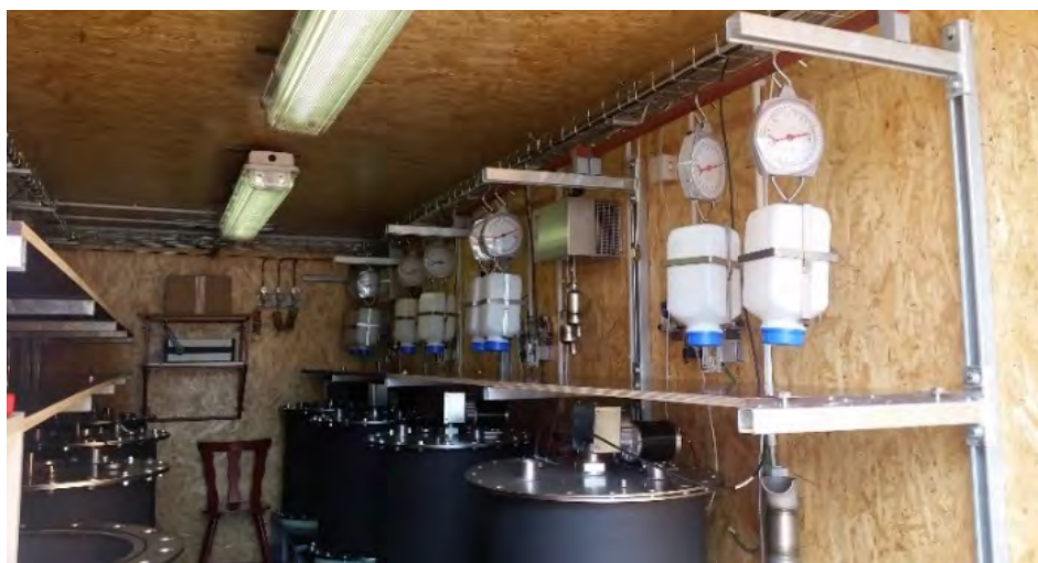
Laboratory container for hydrogen injection experiments (Lecker, 2016)
