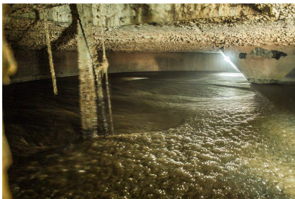
Mixing trials at the full-scale research biogas plant of the University of Hohenheim to evaluate different mixing set-ups (Ohnmacht, 2018)
