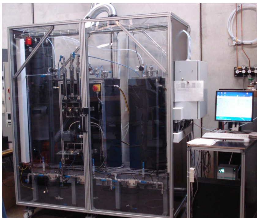
Facility at laboratory scale for fermentative high-pressure methanation of hydrogen and carbon-dioxide
