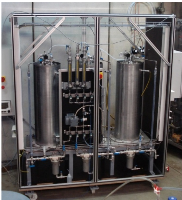
Facility at laboratory scale for fermentative high-pressure methanation of hydrogen and carbon-dioxide
