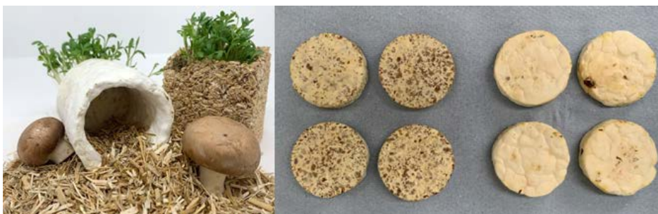
Left: Mycelium-based packaging materials made of hemp shives. Right: Produced samples for further materials testing.
