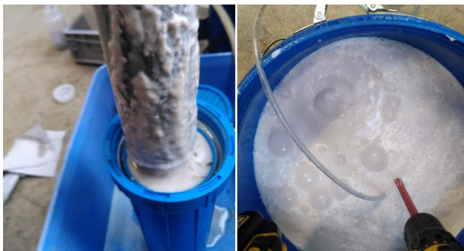
Substrate preparation: Filtration (left) and mixing (right) of the dairy wastewater
